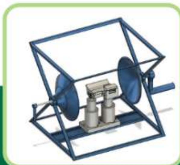
Frontview of Jackfruit Peeling Machine
